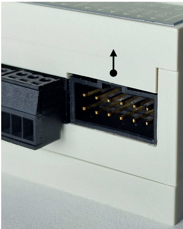
Figure 4: GPIO header location and pinout
