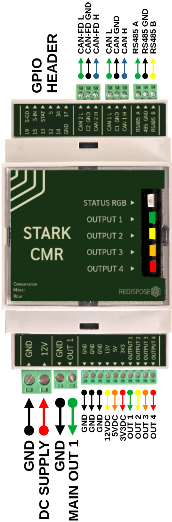
Figure 5: Connector overview and pinout
